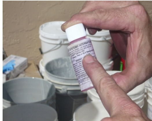
#6 Pour ½ vial of catalyst into ONE of the pails. Use more for faster cure, none or less to slow down the cure time.
